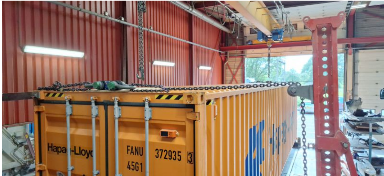
Figure 4-9: Container stiffness tests
